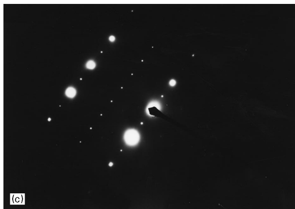
Figure 16 APDs of \text{Ni}_3\text{Al} in melt-spun Ni–Al alloy containing 85 at % Ni: (a) dark-field image of a \text{Ni}_3\text{Al} -grain using an ordered diffraction (b); (c) two SAED patterns, L1_2 [001] and [012] zone, respectively.
